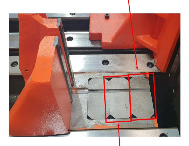
For parts smaller then 20mm you must also remove the second plate
